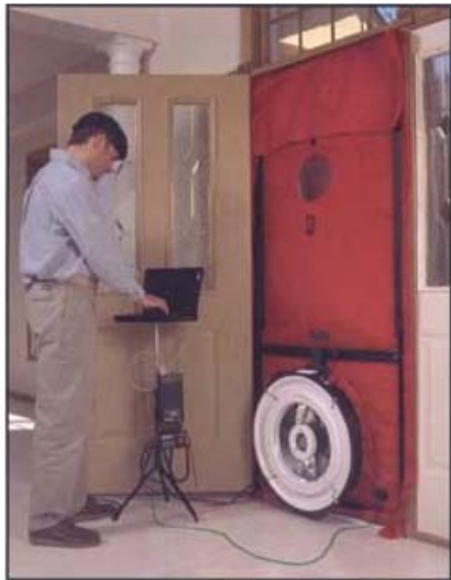
Home Energy Rater performs a blower door test.
